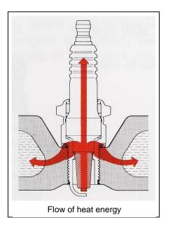
Heat energy transfer is mainly via the threads and sealing area taper (conical seat plugs) or gasket. As a plug is tightened, the threads of the spark plug, and cylinder head are mated and the respective surfaces come into contact. The more a plug is tightened, the more effective the thread contact and sealing areas become (as the gasket flattens). When tightened to within the recommended torque range, rate of heat transfer from the plug through the threads and sealing area is sufficient.
