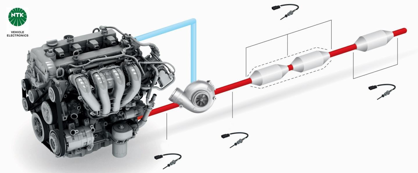
Exhaust Gas Temperature sensors can be utilised in multiple positions on modern vehicle exhaust systems.
